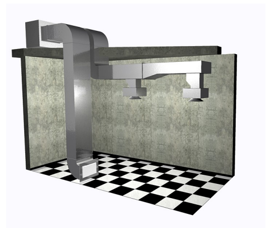
Duct with silencing boxes
